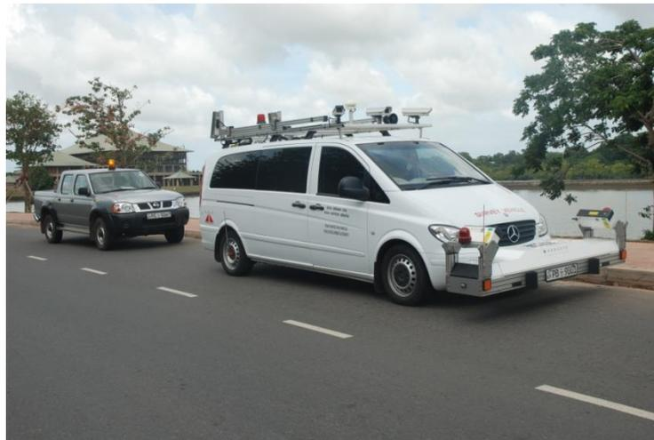
Figure 5-2: Multi-Function Network Survey Vehicle (MFNSV)
