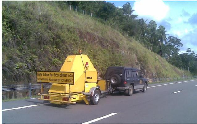
Figure 5-1: Falling Weight Deflectometer (FWD) machine
